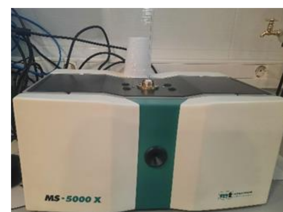
Electron paramagnetic resonance (EPR) instrument used for the antioxidant capacity analysis
